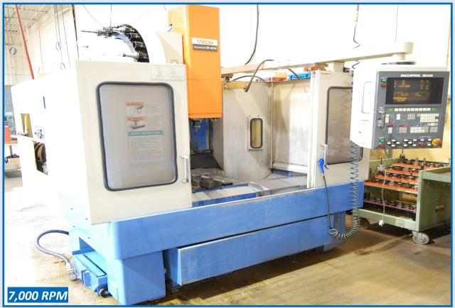
MAZAK MAZATECH MODEL V-414 VERTICAL CNC MACHINING CENTER, S/N 106247, MAZATROL M32B CONTROL, TRAV-ELS: X-22", Y-16.1", Z-18.1", 24 ATC, 7,000 RPM, 35.4" X 16.1" TABLE, 40 TAPER
