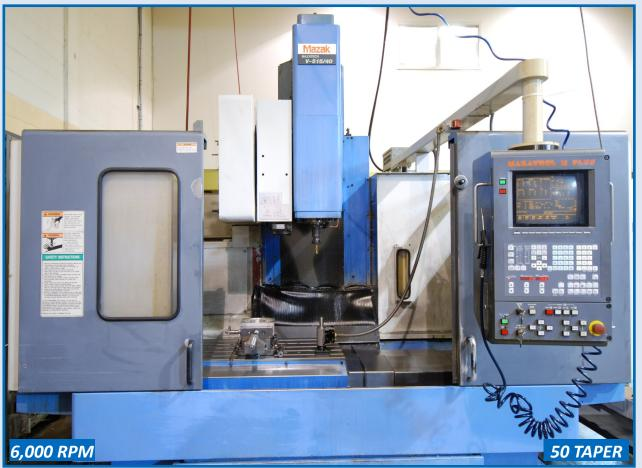
MAZAK MAZATECH MODEL V-515/40 VERTICAL CNC MACHINING CENTER, S/N 118096, MAZATROL M PLUS CONTROL, TRAVELS: X-41.33", Y-20.07", Z-22.04", 30 ATC, 6,000 RPM, 51.18" X 21.65" TABLE, 50 TAPER
